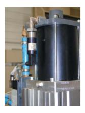
**Analog pressure sensor:** This assembly only allows welding cycle to be triggered when requested force is reached.
