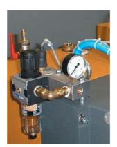
Manual pressure adjustment: In standard version on MA, MC and MB machines.
